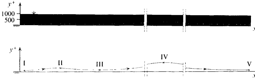
FIGURE 3. Typical particle path recorded by the moving camera system. Particle A . Exposures are spaced 0.087 s apart. I, y^+ = 36 ; II, y^+ = 107 ; III, y^+ = 71 ; IV, y^+ = 338 ; V, y^+ = 80 . Note that the particle images are accurately recorded in the y direction but not in the x direction.
